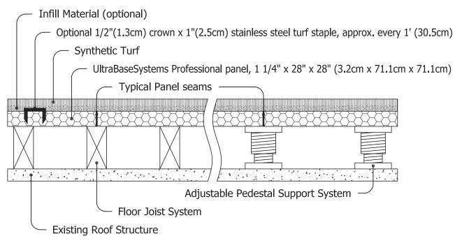
Panel seams must always be supported by Floor Joist/Pedestals, but spacing is dependent upon panel selection and desired rigidity of panel surface
