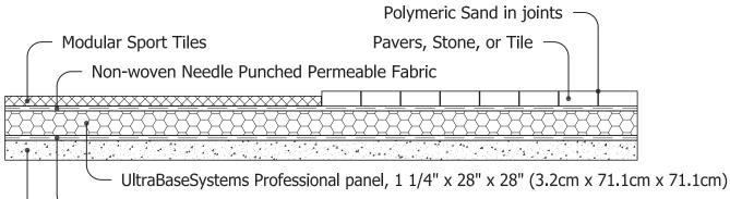
— UltraBaseSystems Geosynthetic Stabilization Fabric
