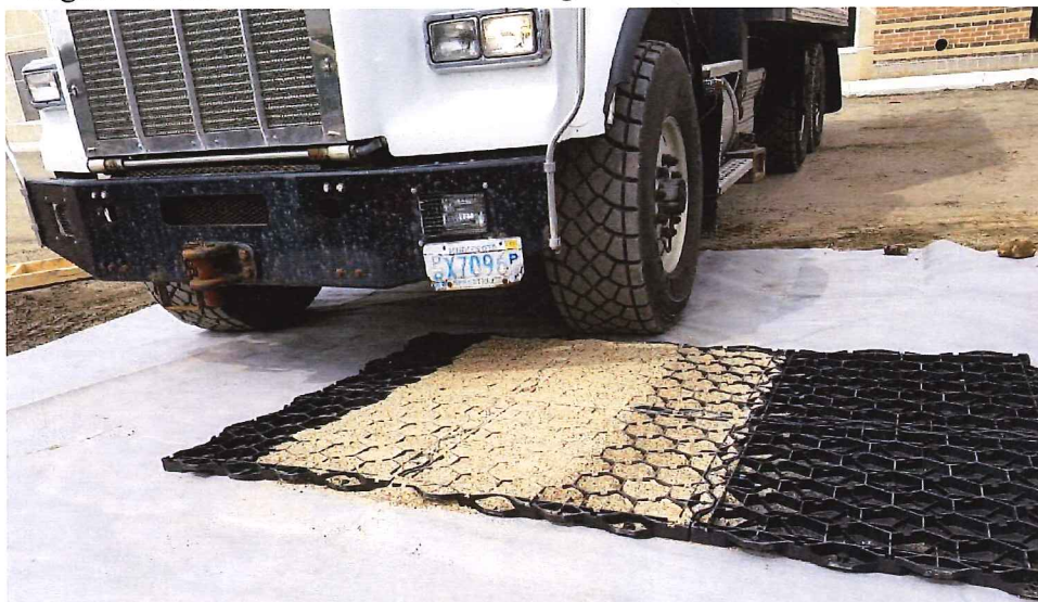
Figure 4: Wheel Load Across the Longitudinal & Transverse Panel Joint
